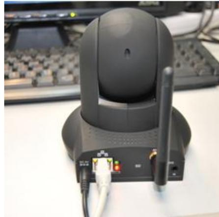
Figure 1.2 – Plug in the network cable
