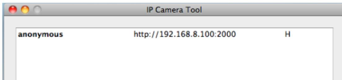
**Figure 2.4 – Static IP address and port 2000 set in IP Camera Tool**
